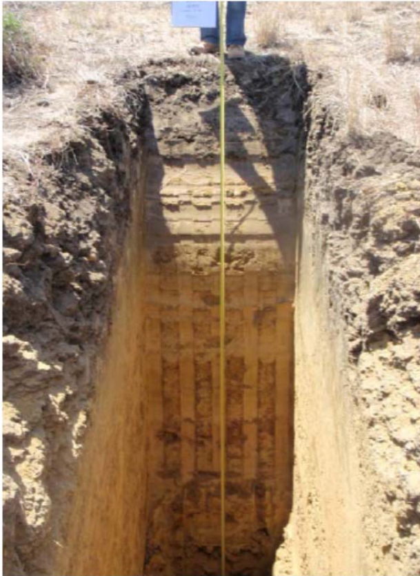
Photo 2 Soil Type 6.2 encountered at KP 170.75 (MLTP095) (Coffey Geotechnics 2008)
