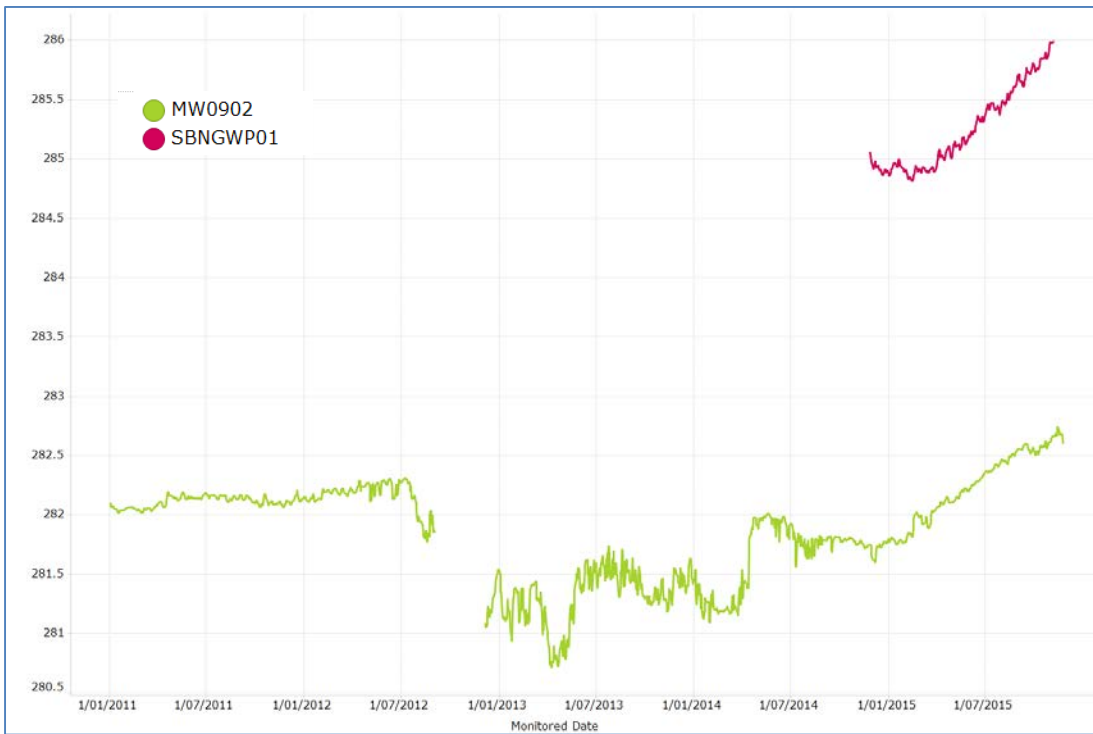
Figure 3-1: Yebna 2 EWS Groundwater Pressure Data
