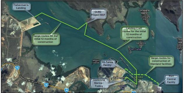
Figure 2-1 Marine facilities and vessel routes for Phase I Construction
